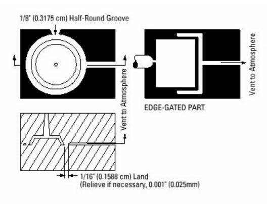
Figure 3-7. Continuous Venting Techniques.
